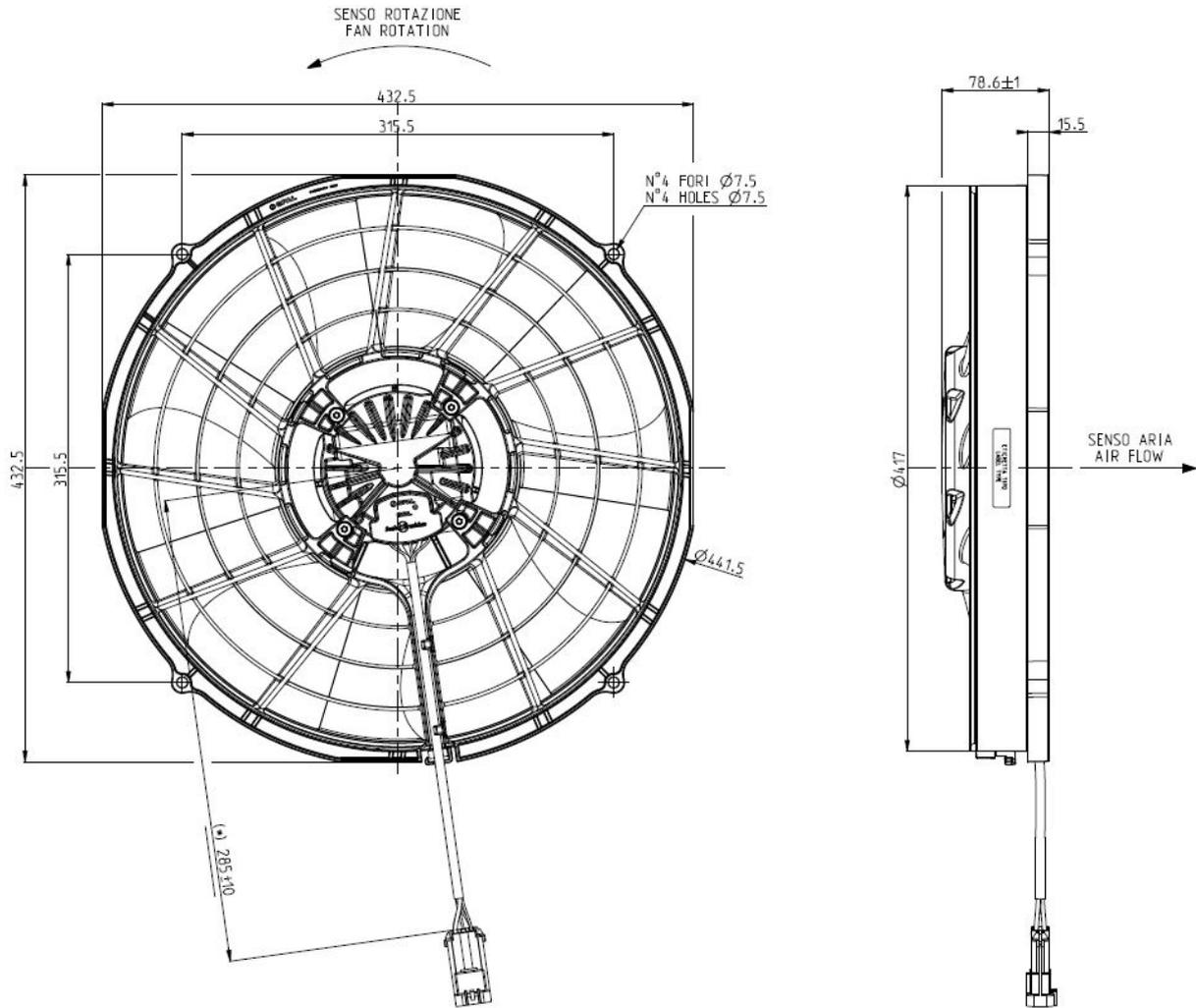
Fixing recommendation: use M6 bolts for fixing. Nominal tightening torque 5 +1/0 Nm
