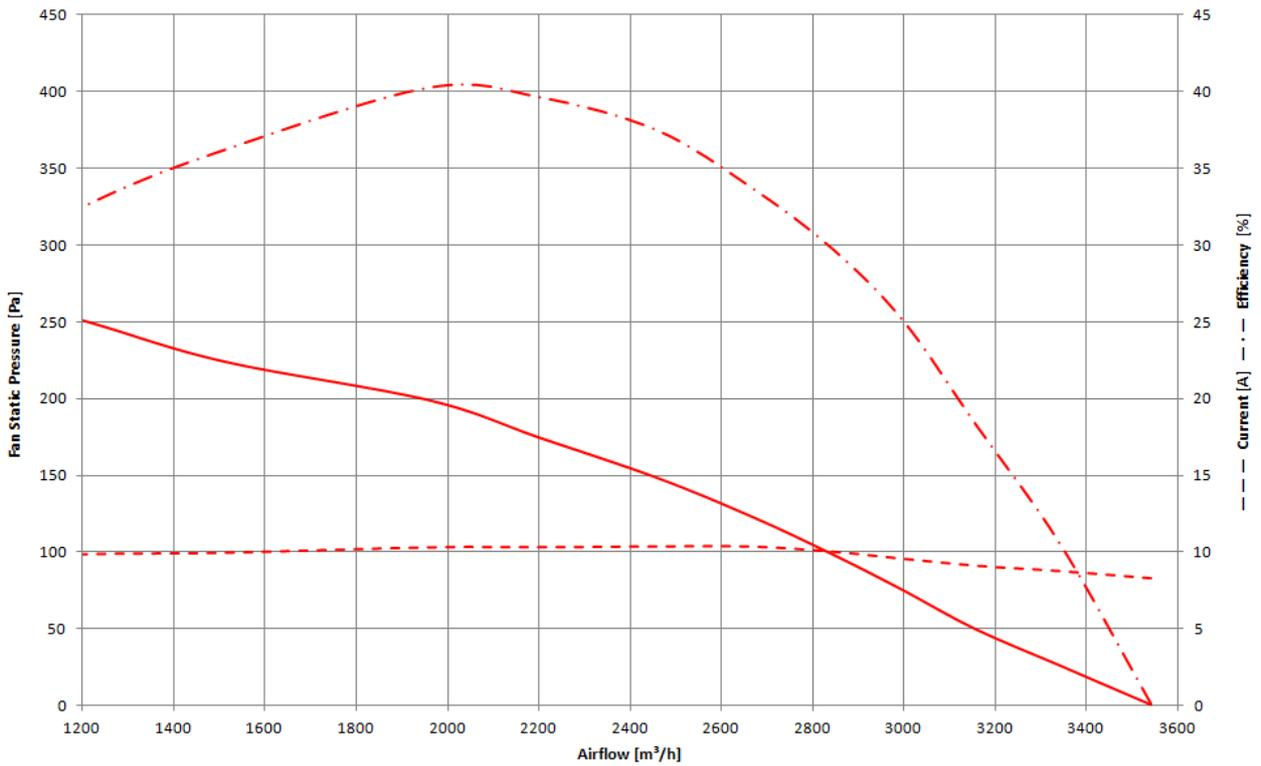
Air density 1.18 kg / m3 - Test number: #15009 – Test bench compliant to ANSI AMCA 210
